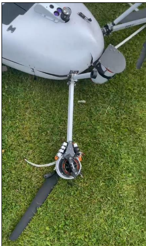
Photo No. 5: Damage to plastic outer shell and missing propeller blades (UA inverted)
