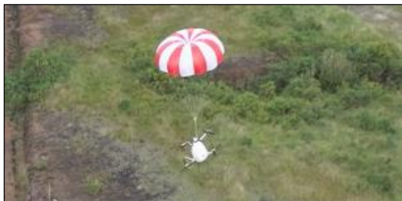
Photo No. 7: Still image of parachute deployment
